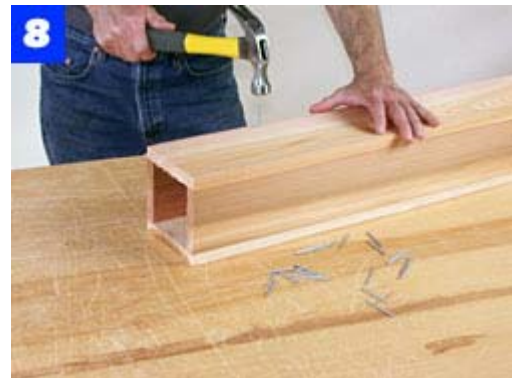
Assemble the box posts with plates but no glue. Then, use galvanized finishing nails to fasten the pieces together.
