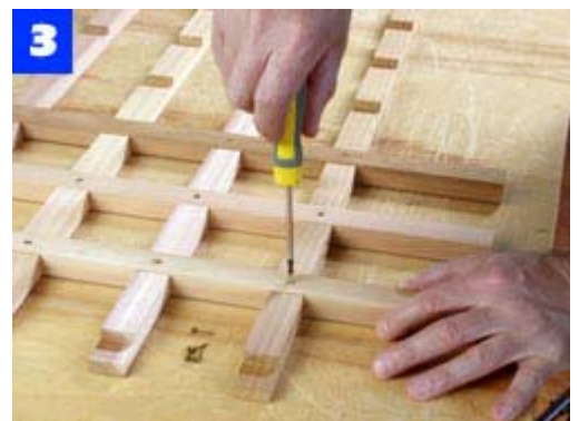
Apply glue to the half-lap joints and press the lattice strips together. Reinforce each joint with a single screw.
