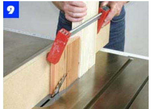
Use a tall auxiliary fence when cutting the post cap angles. Clamp stock to a backer board to support the cut.
