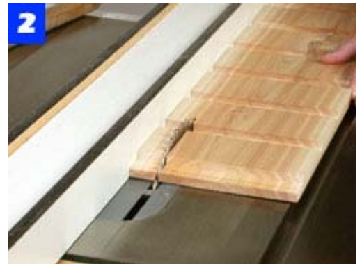
When the notches are cut, rip the 1-in.-wide horizontal and vertical lattice strips from the 1 x 8 blanks.
